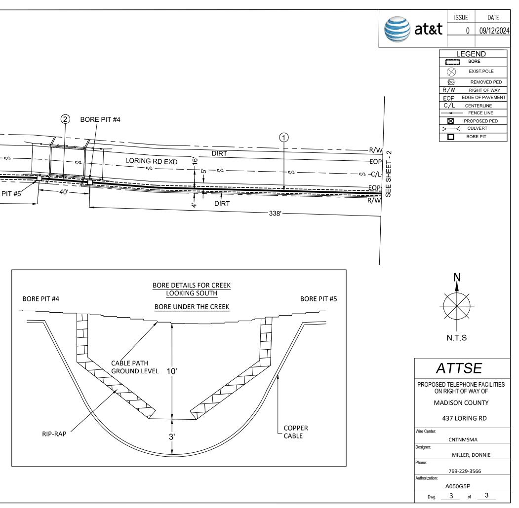
NOTE: BACKFILL & RESTORE THE DIRT SURFACES AS PER COUNTY STANDARDS.
